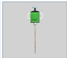
Disposable biopsy needle with Wireless tilting sensor
